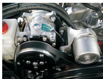
141805 Sanden /R4 multi-groove conversion bracket
